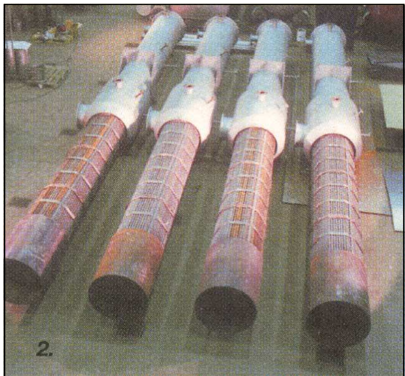
Four twisted tube heat exchangers to be installed in a power plant in China.
