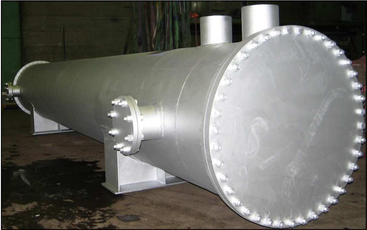
A twisted tube heat exchanger delivered to a power plant in central Sweden.
